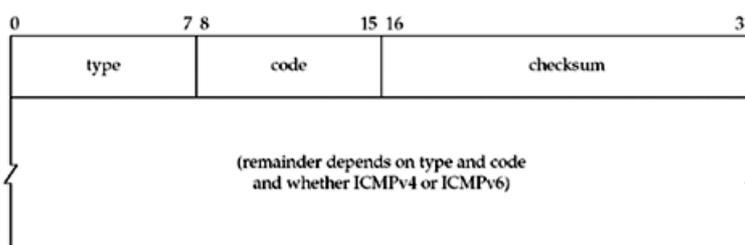
The 8-bit *type* is the type of the ICMPv4 or ICMPv6 message and some types have an 8-bit *code* with additional information. The *checksum* is the standard Internet checksum, although in ICMPv4, the checksum covers only the ICMP payload starting with the type field, while the ICMPv6 checksum also includes the IPv6 pseudoheader.
