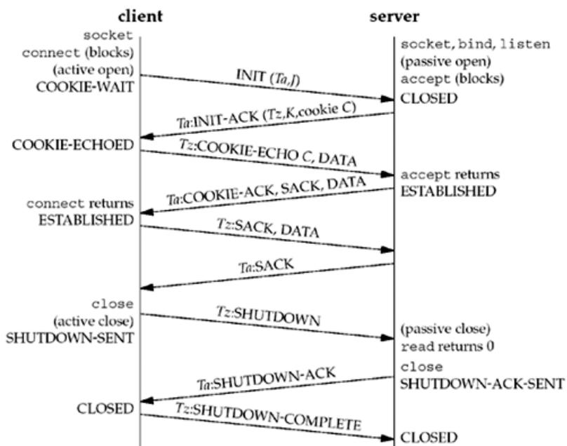
In this example, the client piggybacks its first data chunk on the COOKIE ECHO, and the server replies with data on the COOKIE ACK. In general, the COOKIE ECHO will often have one or more DATA chunks bundled with it when the application is using the one-to-many interface style (we will discuss the one-to-one and one-to-many interface styles in [Section 9.2](#)).
