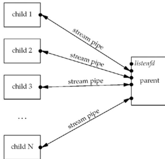
[Figure 30.24](#) shows the `main` function. The changes from previous versions of this function are that descriptor sets are allocated and the bits corresponding to the listening socket along with the stream pipe to each child are turned on in the set. The maximum descriptor value is also calculated. We allocate memory for the array of `Child` structures. The main loop is driven by a call to `select`.
