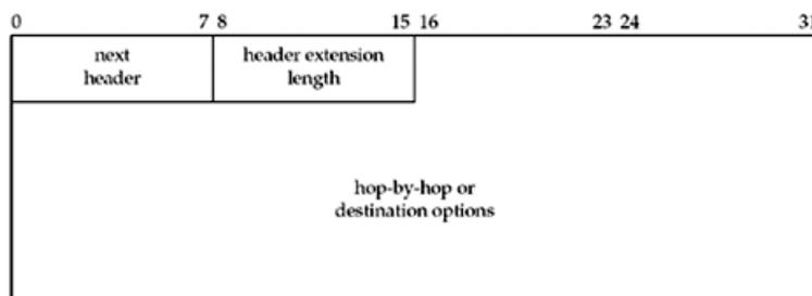
The hop-by-hop options header and destination options header each hold any number of individual options, which have the format shown in [Figure 27.8](#).
