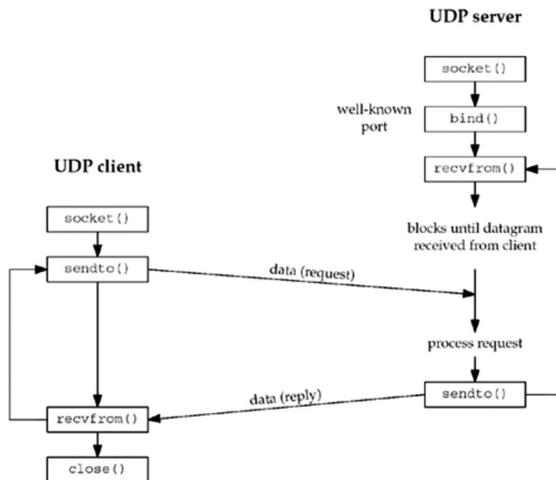
[Figure 8.1](#) shows a timeline of the typical scenario that takes place for a UDP client/server exchange. We can compare this to the typical TCP exchange that was shown in [Figure 4.1](#).
