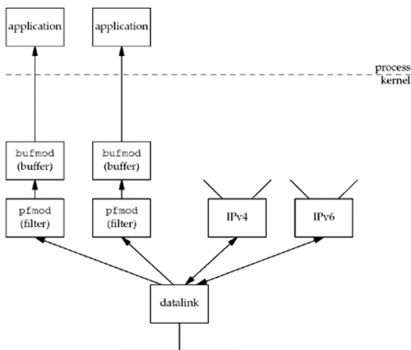
Conceptually, this is similar to what we described in the previous section for BPF: `pfmod` supports filtering within the kernel using a pseudomachine and `bufmod` reduces the amount of data and number of system calls by supporting a snapshot length and a read timeout.
