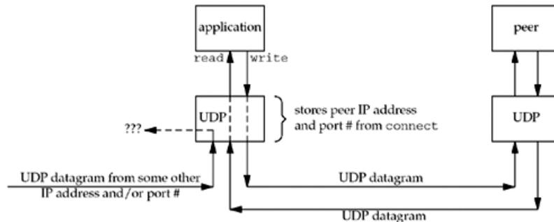
The application calls `connect`, specifying the IP address and port number of its peer. It then uses `read` and `write` to exchange data with the peer.
