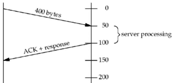
**7.11** Section 4.2.3.2 states: "The delay MUST be less than 0.5 seconds, and in a stream of full-sized segments, there SHOULD be an ACK for at least every second segment." Berkeley-derived implementations delay an ACK by at most 200 ms (p.821 of TCPv2).
