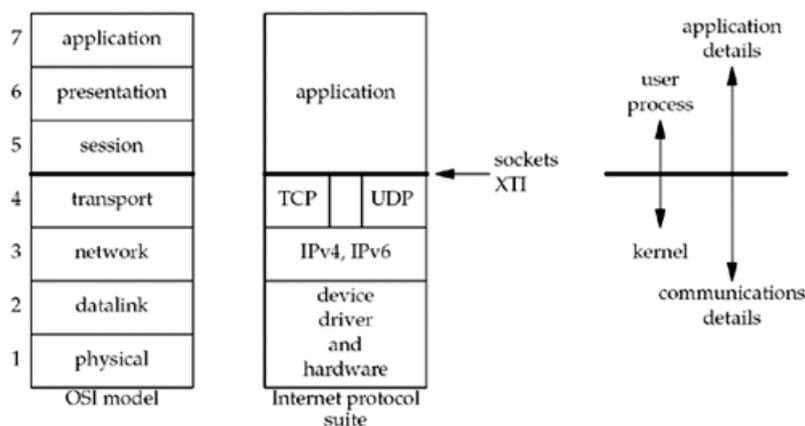
We consider the bottom two layers of the OSI model as the device driver and networking hardware that are supplied with the system. Normally, we need not concern ourselves with these layers other than being aware of some properties of the datalink, such as the 1500-byte Ethernet maximum transfer unit (MTU), which we describe in [Section 2.11](#).
