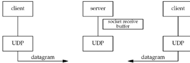
There is only one server process and it has a single socket on which it receives all arriving datagrams and sends all responses. That socket has a receive buffer into which all arriving datagrams are placed.
