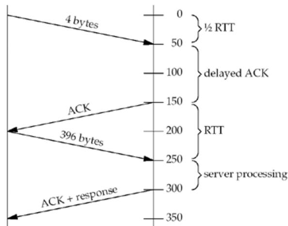
**7.9** Setting the `TCP_NODELAY` socket option causes the data from the second `write` to be sent immediately, even though the connection has a small packet outstanding. We show this in [Figure E.7](#). The total time in this example is just over 150 ms.
