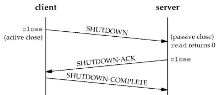
SCTP does not have a `TIME_WAIT` state like TCP, due to its use of verification tags. All chunks are tagged with the tag exchanged in the INIT chunks; a chunk from an old connection will arrive with an incorrect tag. Therefore, in lieu of keeping an entire connection in `TIME_WAIT`, SCTP instead places verification tag values in `TIME_WAIT`.
