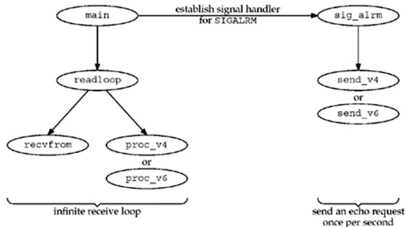
The program operates in two parts: One half reads everything received on a raw socket, printing the ICMP echo replies, and the other half sends an ICMP echo request once per second. The second half is driven by a `SIGALRM` signal once per second.
