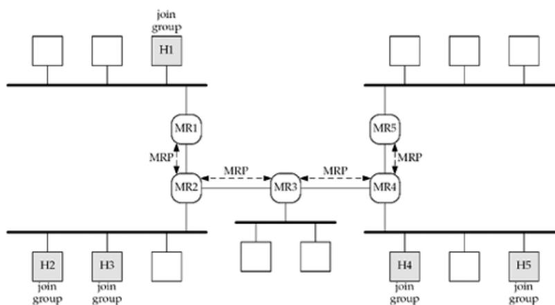
When a process on a host joins a multicast group, that host sends an IGMP message to any attached multicast routers telling them that the host has just joined that group. The multicast routers then exchange this information using the MRP so that each multicast router knows what to do if it receives a packet destined to the multicast address.
