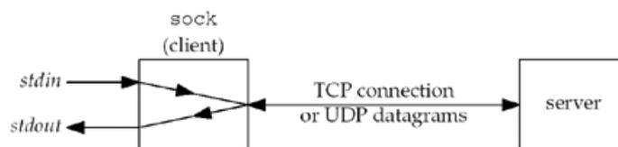
In the client mode, everything read from standard input is written to the network, and everything received from the network is written to standard output. The server's IP address and port must be specified, and in the case of TCP, an active open is performed.
