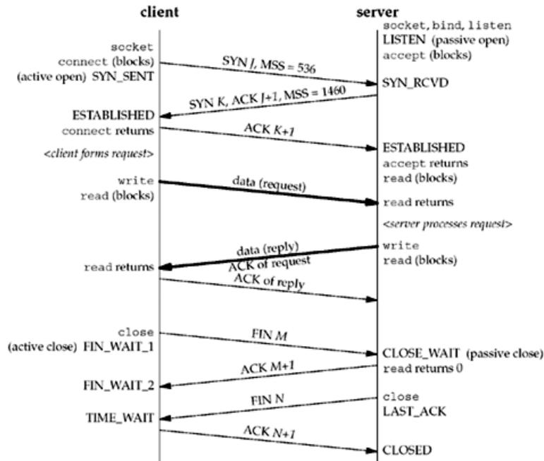
The client in this example announces an MSS of 536 (indicating that it implements only the minimum reassembly buffer size) and the server announces an MSS of 1,460 (typical for IPv4 on an Ethernet). It is okay for the MSS to be different in each direction (see [Exercise 2.5](#)).
