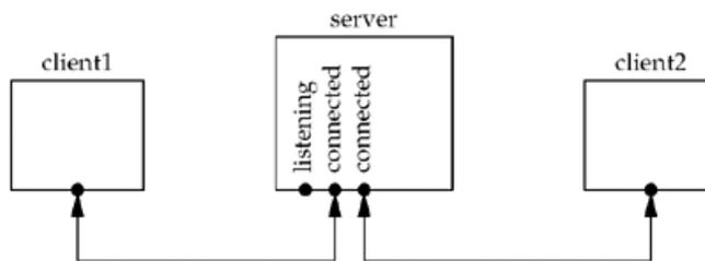
The new connected socket (which we assume is 5) must be remembered, giving the data structures shown in [Figure 6.19](#).
