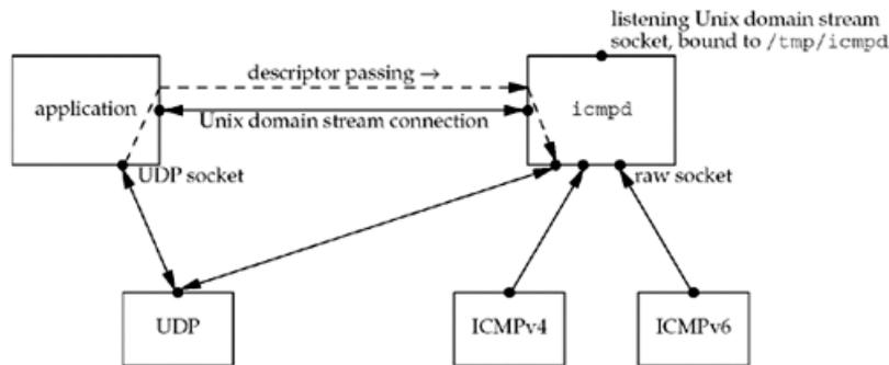
After the daemon obtains the port number bound to the UDP socket, it closes its copy of the socket, taking us back to the arrangement shown in [Figure 28.27](#).
