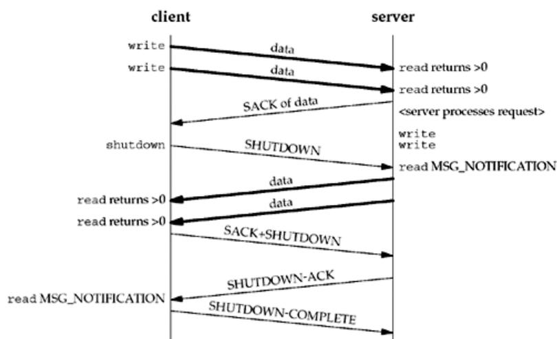
Note that in [Figure 9.5](#), we depict the user receiving the `MSG_NOTIFICATION` events. If the user had not subscribed to receive these events, then a read of length 0 would have been returned. The effects of the `shutdown` function for TCP were described in [Section 6.6](#). The `shutdown` function *howto* holds the following semantics for SCTP:
