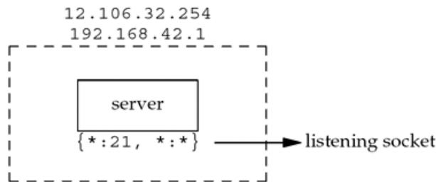
We use the notation `{*:21, *: *}` to indicate the server's socket pair. The server is waiting for a connection request on any local interface (the first asterisk) on port 21. The foreign IP address and foreign port are not specified and we denote them as `*:*`. We also call this a *listening socket*.
