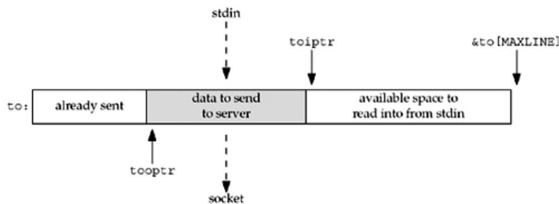
The pointer `toiptr` points to the next byte into which data can be read from standard input. `tooptr` points to the next byte that must be written to the socket. There are `toiptr` minus `tooptr` bytes to be written to the socket. The number of bytes that can be read from standard input is `&to [MAXLINE]` minus `toiptr`. As soon as `tooptr` reaches `toiptr`, both pointers are reset to the beginning of the buffer.
