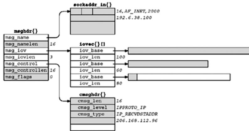
The shaded fields are modified by `recvmsg`. The following items have changed from [Figure 14.8](#) to [Figure 14.9](#):
