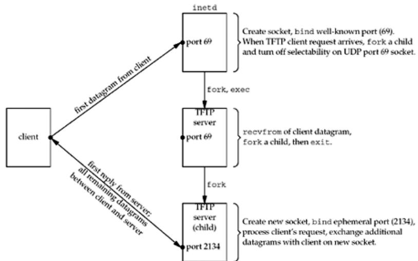
The TFTP server that is the child of `inetd` calls `recvfrom` and reads the client request. It then `forks` a child of its own, and that child will process the client request. The TFTP server then calls `exit`, sending `SIGCHLD` to `inetd`, which tells `inetd` to again `select` on the socket bound to UDP port 69.
