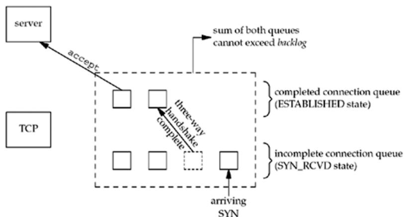
When an entry is created on the incomplete queue, the parameters from the listen socket are copied over to the newly created connection. The connection creation mechanism is completely automatic; the server process is not involved. [Figure 4.8](#) depicts the packets exchanged during the connection establishment with these two queues.
