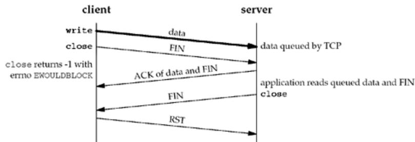
The basic principle here is that a successful return from `close`, with the `SO_LINGER` socket option set, only tells us that the data we sent (and our `FIN`) have been acknowledged by the peer TCP. This does *not* tell us whether the peer application has read the data. If we do not set the `SO_LINGER` socket option, we do not know whether the peer TCP has acknowledged the data.
