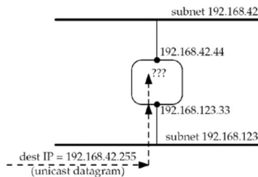
The router receives a unicast IP datagram on the 192.168.123/24 subnet with a destination address of 192.168.42.255 (the subnet-directed broadcast address of another interface). The router normally does not forward the datagram on to the 192.168.42/24 subnet. Some systems have a configuration option that allows subnet-directed broadcasts to be forwarded (Appendix E of TCPv1).
