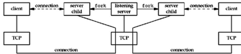
There are two connected sockets and each of the two connected sockets on the server host has its own socket receive buffer.
