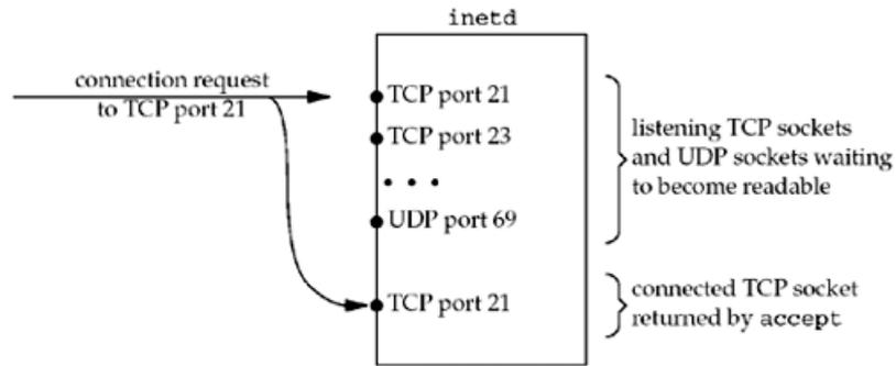
The connection request is directed to TCP port 21, but a new connected socket is created by `accept`.
