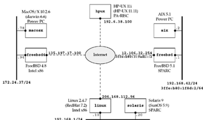
The notation "/24" indicates the number of consecutive bits starting from the leftmost bit of the address used to identify the network and subnet. [Section A.4](#) will talk about the /n notation used today to designate subnet boundaries.
