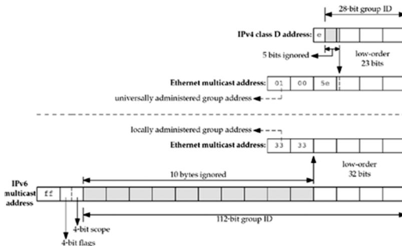
Considering just the IPv4 mapping, the high-order 24 bits of the Ethernet address are always 01:00:5e. The next bit is always 0, and the low-order 23 bits are copied from the low-order 23 bits of the multicast group address. The high-order 5 bits of the group address are ignored in the mapping. This means that 32 multicast addresses map to a single Ethernet address: The mapping is not one-to-one.
