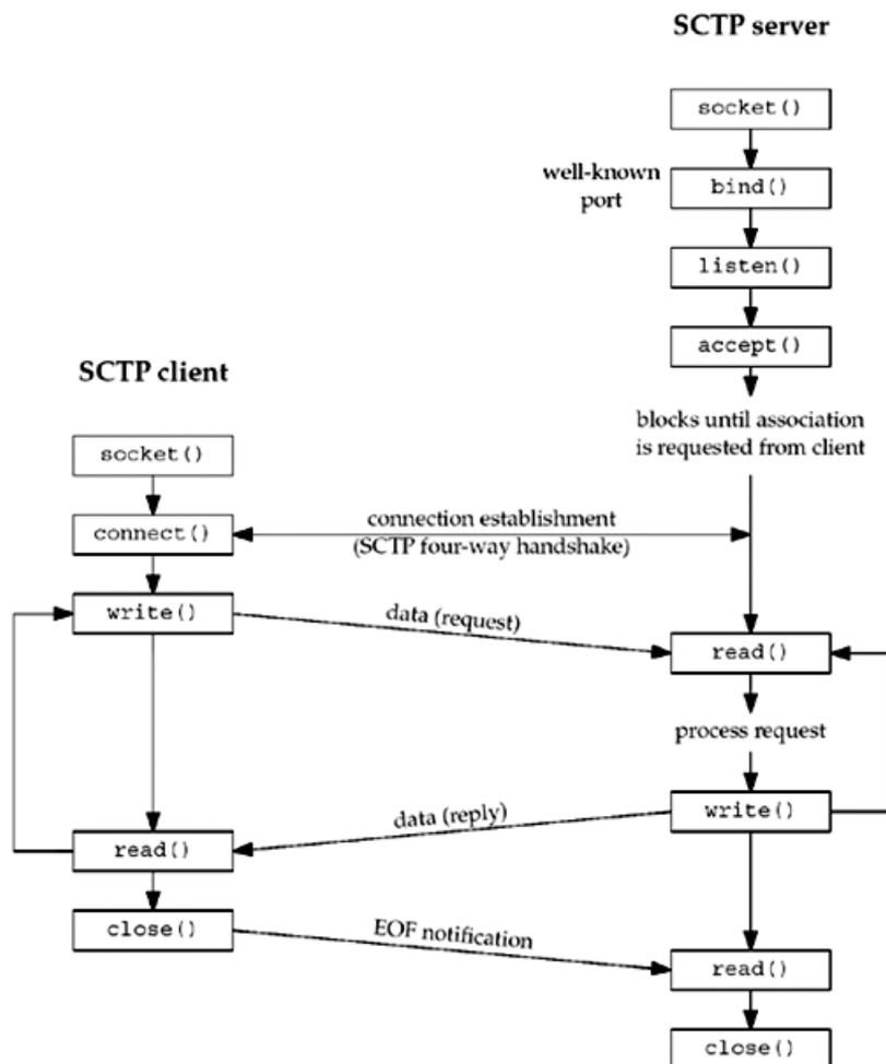
A one-to-one-style SCTP socket is an IP socket (family `AF_INET` or `AF_INET6`), with type `SOCK_STREAM` and protocol `IPPROTO_SCTP`.
