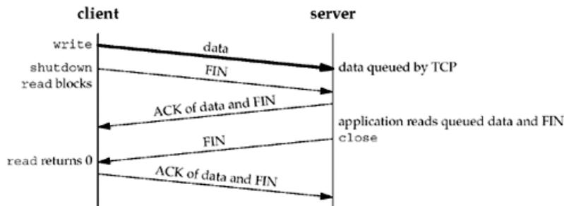
Comparing this figure to [Figures 7.7](#) and [7.8](#) we see that when we close our end of the connection, depending on the function called (`close` or `shutdown`) and whether the `SO_LINGER` socket option is set, the return can occur at three different times:
