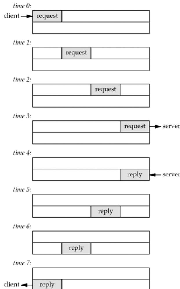
A request is sent by the client at time 0 and we assume an RTT of 8 units of time. The reply sent at time 4 is received at time 7. We also assume that there is no server processing time and that the size of the request is the same as the reply. We show only the data packets between the client and server, ignoring the TCP acknowledgments that are also going across the network.
