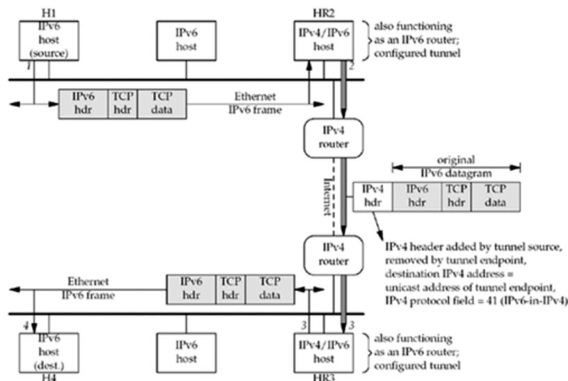
1. Host H1 on the top LAN sends an IPv6 datagram containing a TCP segment to host H4 on the bottom LAN. We designate these two hosts as "IPv6 hosts," but both probably run IPv4 also. The IPv6 routing table on H1 specifies that host HR2 is the next-hop router and an IPv6 datagram is sent to this host.
