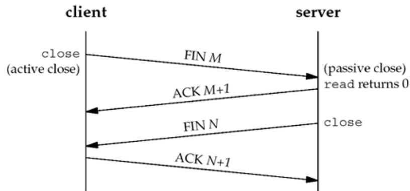
A FIN occupies one byte of sequence number space just like a SYN. Therefore, the ACK of each FIN is the sequence number of the FIN plus one.
