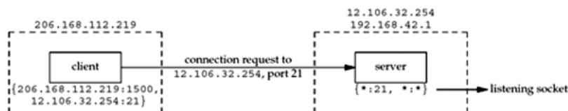
When the server receives and accepts the client's connection, it `forks` a copy of itself, letting the child handle the client, as we show in [Figure 2.13](#). (We will describe the `fork` function in [Section 4.7](#).)
