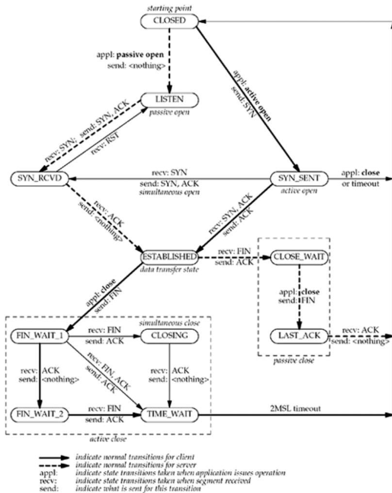
There are 11 different states defined for a connection and the rules of TCP dictate the transitions from one state to another, based on the current state and the segment received in that state. For example, if an application performs an active open in the CLOSED state, TCP sends a SYN and the new state is SYN\_SENT. If TCP next receives a SYN with an ACK, it sends an ACK and the new state is ESTABLISHED. This final state is where most data transfer occurs.
