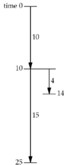
To further optimize this sequence, the client can start parsing the data that is returned for the first connection before the first connection completes and initiate additional connections as soon as it knows that additional connections are needed.
