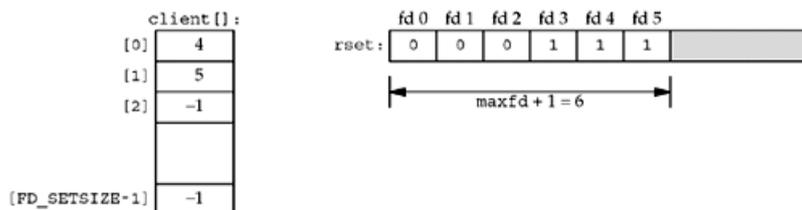
Next, we assume the first client terminates its connection. The client TCP sends a FIN, which makes descriptor 4 in the server readable. When our server reads this connected socket, `read` returns 0. We then close this socket and update our data structures accordingly. The value of `client [0]` is set to `-1` and descriptor 4 in the descriptor set is set to 0. This is shown in [Figure 6.20](#). Notice that the value of `maxfd` does not change.
