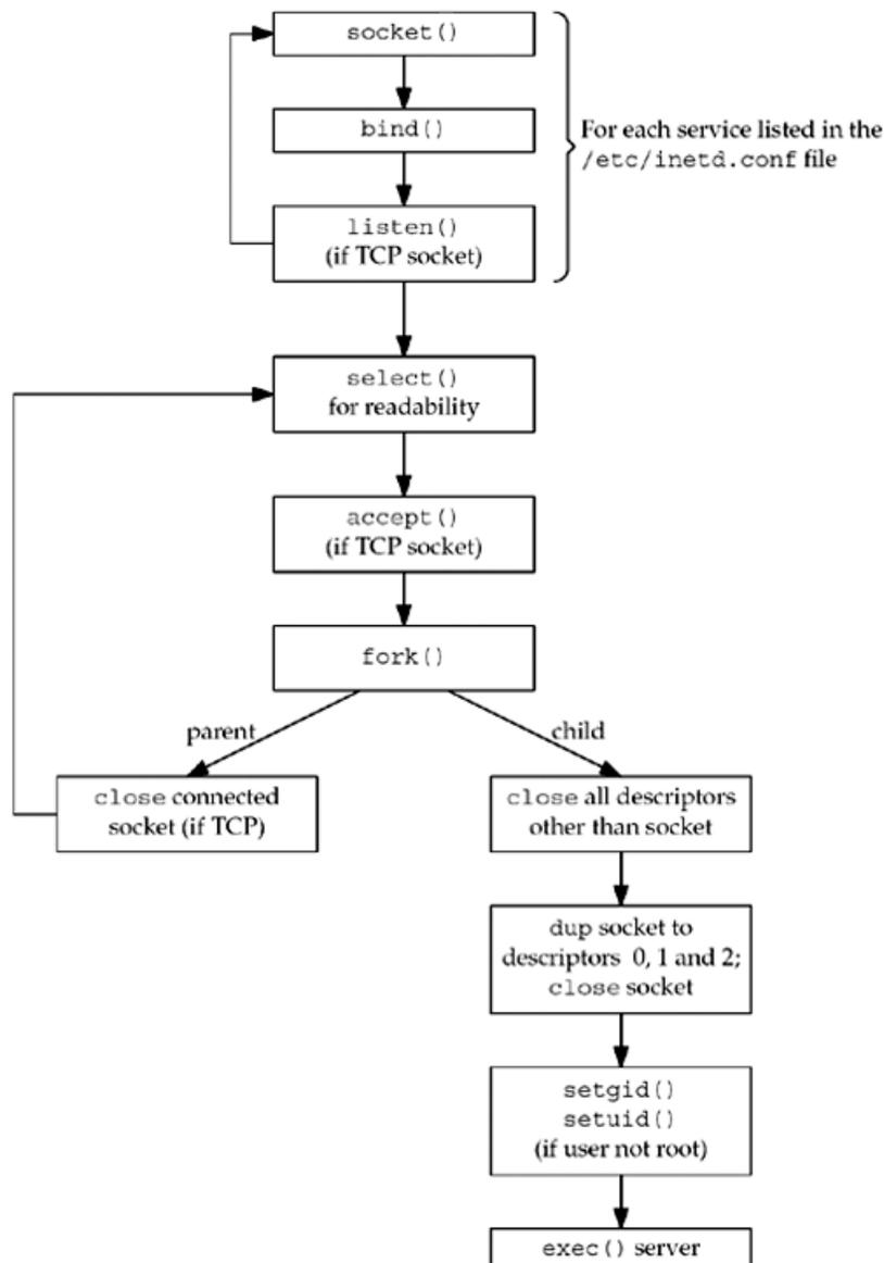
1. On startup, it reads the `/etc/inetd.conf` file and creates a socket of the appropriate type (stream or datagram) for all the services specified in the file. The maximum number of servers that `inetd` can handle depends on the maximum number of descriptors that `inetd` can create. Each new socket is added to a descriptor set that will be used in a call to `select`.
