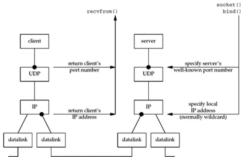
There are at least four pieces of information that a server might want to know from an arriving IP datagram: the source IP address, destination IP address, source port number, and destination port number. [Figure 8.13](#) shows the function calls that return this information for a TCP server and a UDP server.
