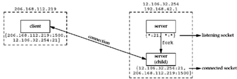
At this point, we must distinguish between the listening socket and the connected socket on the server host. Notice that the connected socket uses the same local port (21) as the listening socket. Also notice that on the multihomed server, the local address is filled in for the connected socket (12.106.32.254) once the connection is established.
