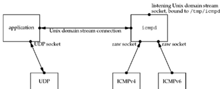
The application next "passes" its UDP socket to the daemon across the Unix domain connection using *descriptor passing*, as we described in [Section 15.7](#). This gives the daemon a copy of the socket so that it can call `getsockname` and obtain the port number bound to the socket. We will show this passing of the socket in [Figure 28.28](#).
