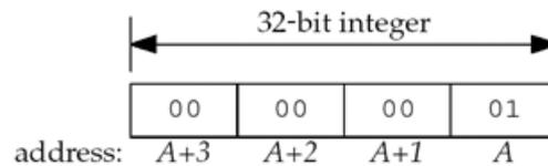
The 4 bytes are sent across the socket in the order  $A$ ,  $A+1$ ,  $A+2$ , and  $A+3$  where they are stored in the big-endian format, as shown in [Figure E.3](#).
