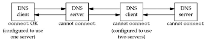
A DNS client can be configured to use one or more servers, normally by listing the IP addresses of the servers in the file `/etc/resolv.conf`. If a single server is listed (the leftmost box in the figure), the client can call `connect`, but if multiple servers are listed (the second box from the right in the figure), the client cannot call `connect`. Also, a DNS server normally handles any client request, so the servers cannot call `connect`.
