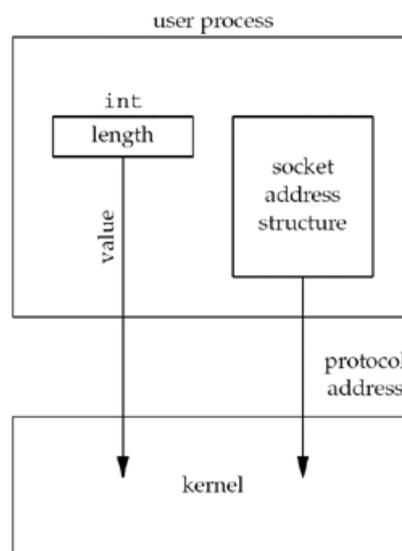
We will see in the next chapter that the datatype for the size of a socket address structure is actually `socklen_t` and not `int`, but the POSIX specification recommends that `socklen_t` be defined as `uint32_t`.
