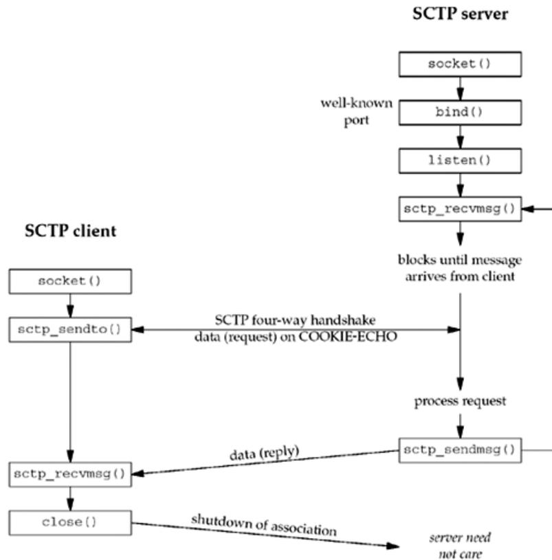
This example shows an iterative server, where (possibly interleaved) messages from many associations (i.e., many clients) can be processed by a single thread of control. With SCTP, a one-to-many socket can also be used in conjunction with the `sctp_peeloff` function (see [Section 9.12](#)) to allow the iterative and concurrent server models to be combined as follows:
