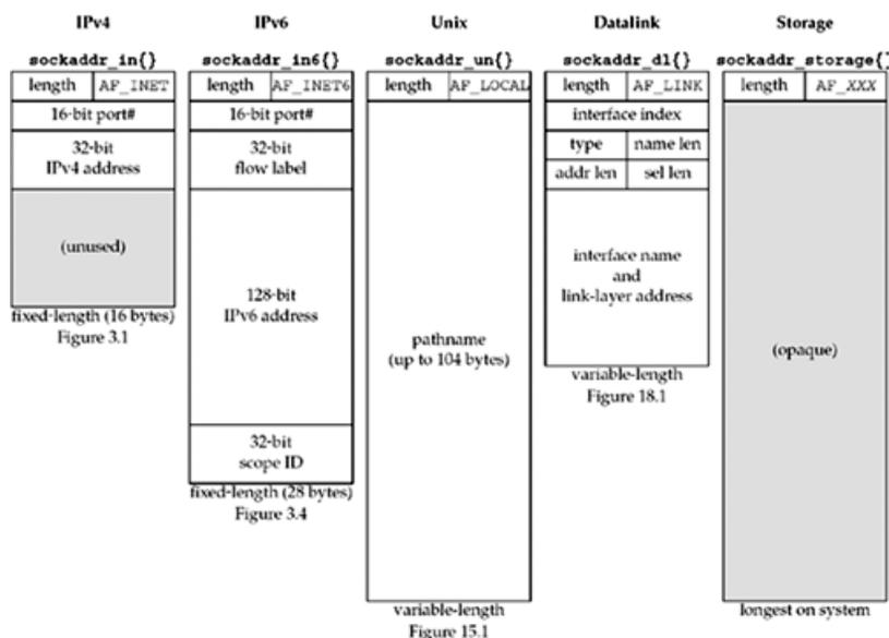
Two of the socket address structures are fixed-length, while the Unix domain structure and the datalink structure are variable-length. To handle variable-length structures, whenever we pass a pointer to a socket address structure as an argument to one of the socket functions, we pass its length as another argument. We show the size in bytes (for the 4.4BSD implementation) of the fixed-length structures beneath each structure.
