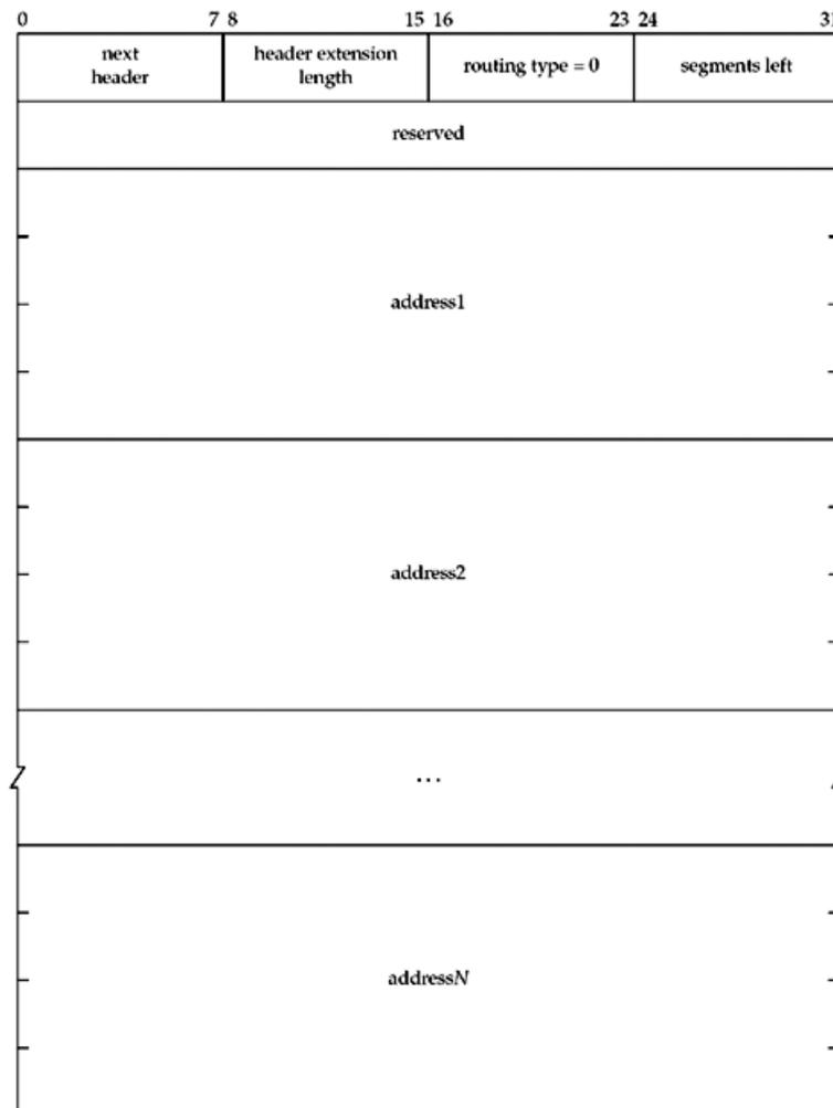
An unlimited number of addresses can appear in the routing header (limited only by packet length) and *segments left* must be equal to or less than the number of addresses in the header. RFC 2460 [Deering and Hinden 1998] specifies the details of how the header is processed as the packet travels to the final destination, along with a detailed example.
