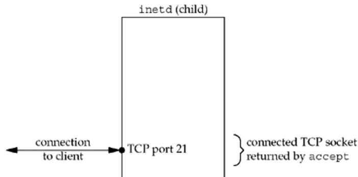
The next step is for the child to duplicate the connected socket to descriptors 0, 1, and 2 and then close the connected socket. This gives us the descriptors shown in [Figure 13.10](#).
