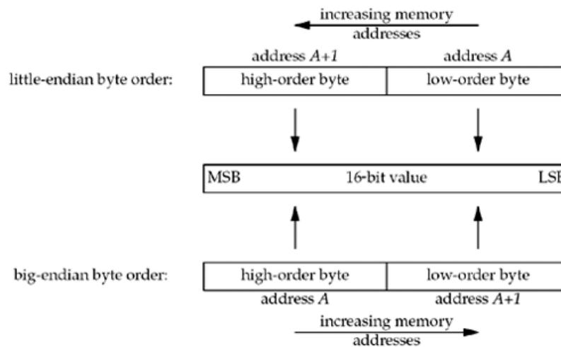
In this figure, we show increasing memory addresses going from right to left in the top, and from left to right in the bottom. We also show the most significant bit (MSB) as the leftmost bit of the 16-bit value and the least significant bit (LSB) as the rightmost bit.
