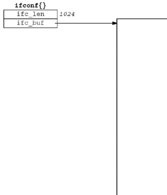
If we assume that the kernel returns two `ifreq` structures, we could have the arrangement shown in [Figure 17.4](#) (p. 470) when the `ioctl` returns. The shaded regions have been modified by `ioctl`. The buffer has been filled in with the two structures and the `ifc_len` member of the `ifconf` structure has been updated to reflect the amount of information stored in the buffer. We assume in this figure that each `ifreq` structure occupies 32 bytes.
