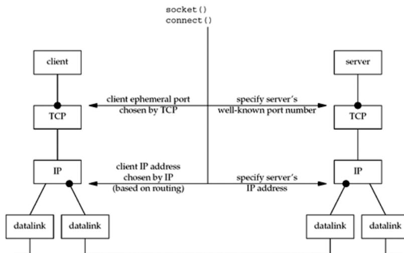
As we mentioned in [Section 4.10](#), the client can obtain the two local values chosen by the kernel by calling `getsockname` after the connection is established.
