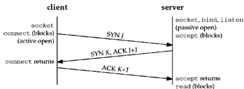
We show the client's initial sequence number as  $J$  and the server's initial sequence number as  $K$ . The acknowledgment number in an ACK is the next expected sequence number for the end sending the ACK. Since a SYN occupies one byte of the sequence number space, the acknowledgment number in the ACK of each SYN is the initial sequence number plus one. Similarly, the ACK of each FIN is the sequence number of the FIN plus one.
