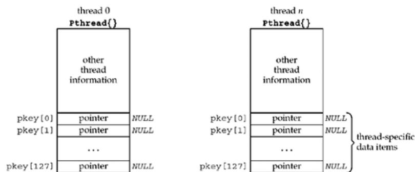
All entries in the `pkey` array are initialized to null pointers. These 128 pointers are the "values" associated with each of the possible 128 "keys" in the process.
