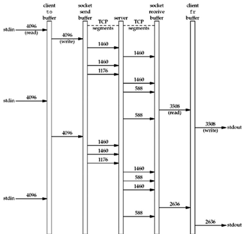
In this figure, we do not show the ACK segments. Also realize that when the program outputs "wrote *N* bytes to stdout," the `write` has returned, possibly causing TCP to send one or more segments of data.
