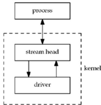
The *stream head* consists of the kernel routines that are invoked when the application makes a system call for a STREAMS descriptor (e.g., `read`, `putmsg`, `ioctl`, and the like).
