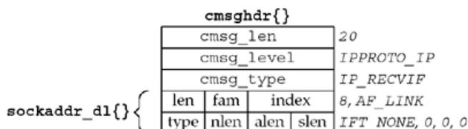
Recall the datalink socket address structure in [Figure 18.1](#). The data returned in the ancillary data object is one of these structures, but the three lengths are 0 (name length, address length, and selector length). Therefore, there is no need for any of the data that follows these lengths, so the size of the structure should be 8 bytes, not the 20 that we show in [Figure 18.1](#). The information we return is the interface index.
