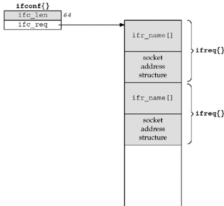
A pointer to an `ifreq` structure is also used as an argument to the remaining interface `ioctl`s shown in [Figure 17.1](#), which we will describe in [Section 17.7](#). Notice that each `ifreq` structure contains a `union` and there are numerous `#defines` to hide the fact that these fields are members of a `union`. All references to individual members are made using defined names. Be aware that some systems have added many implementation-dependent members to the `ifr_ifru` `union`.
