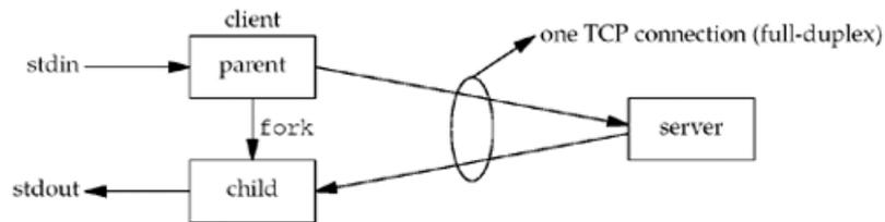
We explicitly note that the TCP connection is full-duplex and that the parent and child are sharing the same socket descriptor: The parent writes to the socket and the child reads from the socket. There is only one socket, one socket receive buffer, and one socket send buffer, but this socket is referenced by two descriptors: one in the parent and one in the child.
