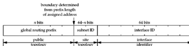
The interface ID must be constructed in modified *EUI-64* format. This is a variation of IEEE *EUI-64* format [IEEE 1997], which is a superset of the 48-bit IEEE 802 MAC addresses that are assigned to most LAN interface cards. This identifier should be automatically assigned for an interface based on its hardware MAC address when possible. Details for constructing
