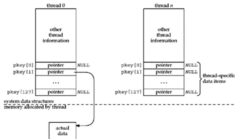
In this figure, we note that the `Pthread` structure is maintained by the system (probably the thread library), but the actual thread-specific data that we `malloc` is maintained by our function (`readline`, in this case). All that `pthread_setspecific` does is set the pointer for this key in the `Pthread` structure to point to our allocated memory. Similarly, all that `pthread_getspecific` does is return that pointer to us.
