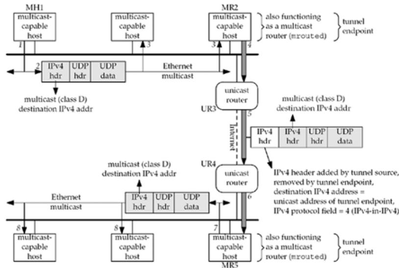
1. An application on the source host, MH1, sends a multicast datagram to a class D address.
