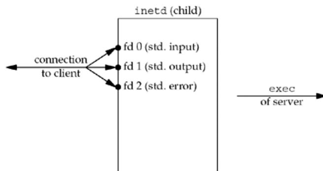
The child then calls `exec`. Recall from [Section 4.7](#) that all descriptors normally remain open across an `exec`, so the real server that is `execed` uses any of the descriptors, 0, 1, or 2, to communicate with the client. These should be the only descriptors open in the server.
