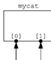
The process then calls `fork` and the child calls `exec` to execute the `openfile` program. The parent closes the `[1]` descriptor and the child closes the `[0]` descriptor. (There is no difference in either end of the stream pipe; the child could close `[1]` and the parent could close `[0]`.) This gives us the arrangement shown in [Figure 15.8](#).
