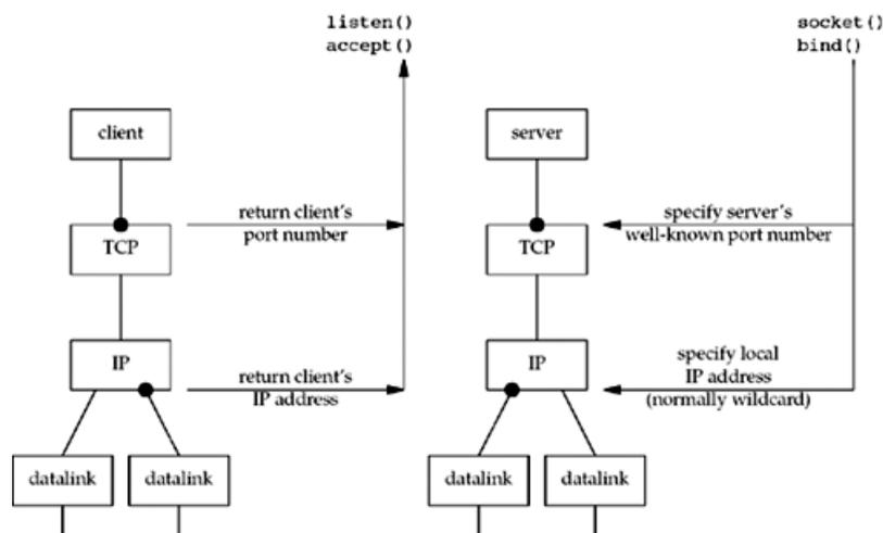
The local port (the server's well-known port) is specified by `bind`. Normally, the server also specifies the wildcard IP address in this call. If the server binds the wildcard IP address on a multihomed host, it can determine the local IP address by calling `getsockname` after the connection is established ([Section 4.10](#)). The two foreign values are returned to the server
