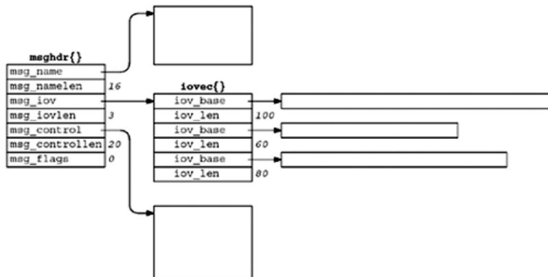
Sixteen bytes are allocated for the protocol address and 20 bytes are allocated for the ancillary data. An array of three `iovec` structures is initialized: The first specifies a 100-byte buffer, the second a 60-byte buffer, and the third an 80-byte buffer. We also assume that the `IP_RECVDSTADDR` socket option has been set for the socket, to receive the destination IP address from the UDP datagram.
