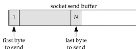
The process now writes a single byte of out-of-band data, containing the ASCII character `a`, using the `send` function and the `MSG_OOB` flag.
