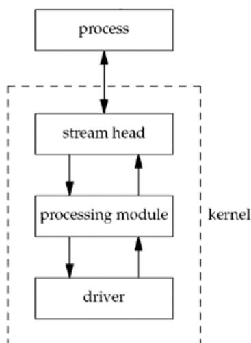
Any number of modules can be pushed onto a stream. When we say "*push*," we mean that each new module gets inserted just below the stream head.
