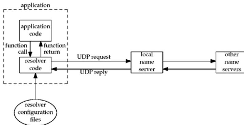
The resolver code reads its system-dependent configuration files to determine the location of the organization's name servers. (We use the plural "name servers" because most organizations run multiple name servers, even though we show only one local server in the figure. Multiple name servers are absolutely required for reliability and redundancy.) The file `/etc/resolv.conf` normally contains the IP addresses of the local name servers.
