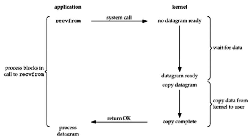
We use UDP for this example instead of TCP because with UDP, the concept of data being "ready" to read is simple: either an entire datagram has been received or it has not. With TCP it gets more complicated, as additional variables such as the socket's low-water mark come into play.
