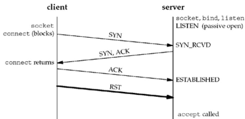
Here, the three-way handshake completes, the connection is established, and then the client TCP sends an RST (reset). On the server side, the connection is queued by its TCP, waiting for the server process to call `accept` when the RST arrives. Sometime later, the server process calls `accept`.
