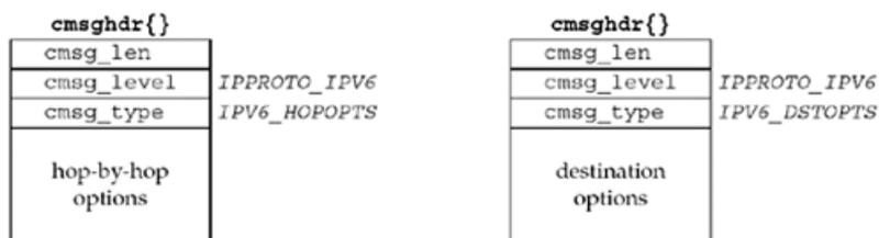
The actual contents of the IPv6 option header is passed between the user and the kernel as the `msg_data` portion of these objects. To reduce code duplication, seven functions are defined to create and process these data sections. The following four functions build an option to send:
