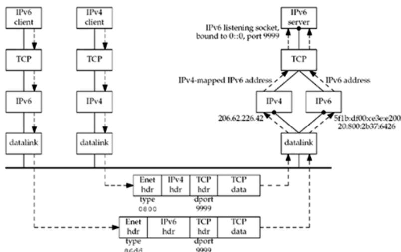
We have an IPv4 client and an IPv6 client on the left. The server on the right is written using IPv6 and it is running on a dual-stack host. The server has created an IPv6 listening TCP socket that is bound to the IPv6 wildcard address and TCP port 9999.
