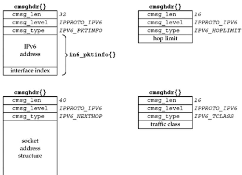
An `in6_pktinfo` structure contains either the source IPv6 address and outgoing interface index for an outgoing datagram or the destination IPv6 address and arriving interface index for a received datagram.
