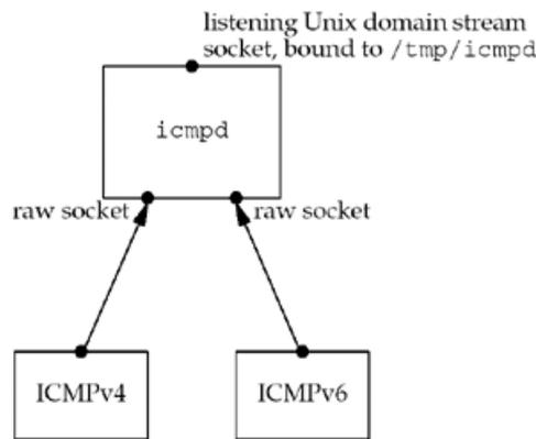
A UDP application (which is a client to the daemon) first creates its UDP socket, the socket for which it wants to receive asynchronous errors. The application must `bind` an ephemeral port to this socket, for reasons we will discuss later. It then creates a Unix domain socket and `connects` to this daemon's well-known pathname. We will show this in [Figure 28.27](#).
