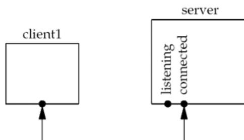
From this point on, our server must remember the new connected socket in its `client` array, and the connected socket must be added to the descriptor set. These updated data structures are shown in [Figure 6.17](#).
