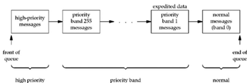
Although the STREAMS system supports 256 different priority bands, networking protocols often use band 1 for expedited data and band 0 for normal data.
