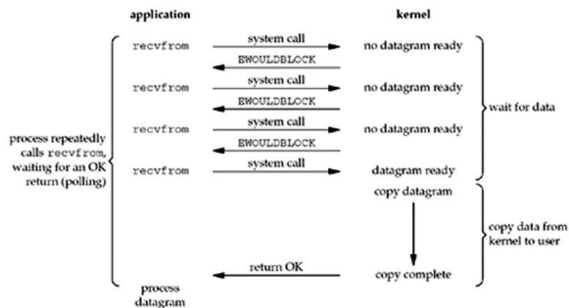
The first three times that we call `recvfrom`, there is no data to return, so the kernel immediately returns an error of `EWOULDBLOCK` instead. The fourth time we call `recvfrom`, a datagram is ready, it is copied into our application buffer, and `recvfrom` returns successfully. We then process the data.
