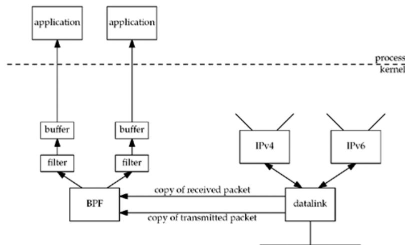
Examples of these calls for an Ethernet interface are in Figures 4.11 and 4.19 of TCPv2. The reason for calling BPF as soon as possible after reception and as late as possible before transmission is to provide accurate timestamps.
