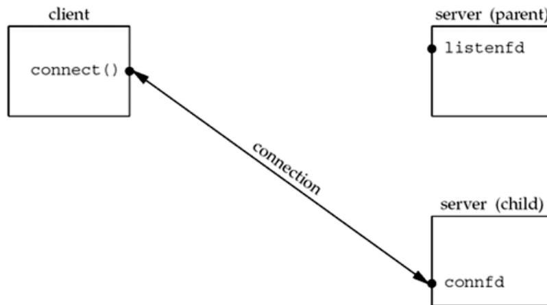
This is the desired final state of the sockets. The child is handling the connection with the client and the parent can call `accept` again on the listening socket, to handle the next client connection.
