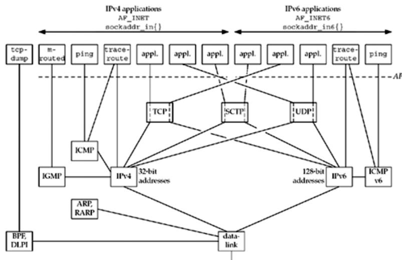
We show both IPv4 and IPv6 in this figure. Moving from right to left, the rightmost five applications are using IPv6; we will talk about the `AF_INET6` constant in [Chapter 3](#), along with the `sockaddr_in6` structure. The next six applications use IPv4.
