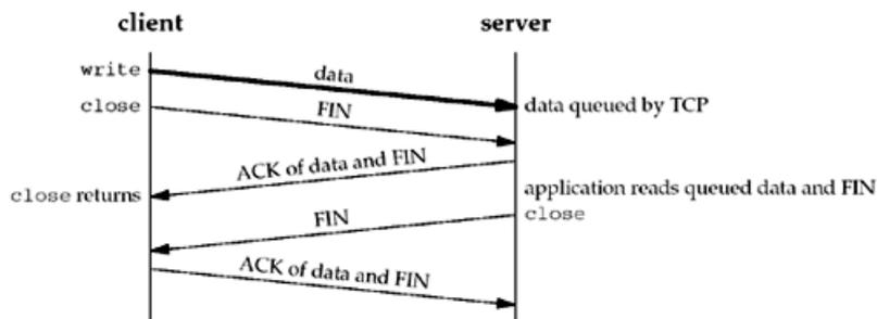
But we still have the same problem as in [Figure 7.7](#): The server host can crash before the server application reads its remaining data, and the client application will never know. Worse, [Figure 7.9](#) shows what can happen when the `SO_LINGER` option is set to a value that is too low.
