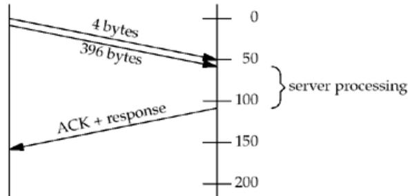
**7.10** The advantage to this solution is reducing the number of packets, as we show in [Figure E.8](#).
